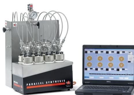
PolyBLOCK 4/8 high pressure parallel automated reactor system
