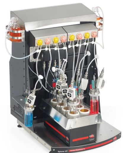
BioXplorer 100 in a typical 8-reactor configuration
