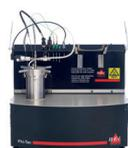
Phi-TEC I calorimeter
