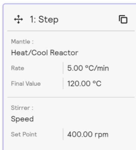
Figure 2. Heat/Cool Reactor step on labCONSOL ® heating by 5 °C/min to 120 °C with a stirring speed of 400 rpm.
